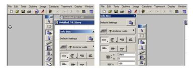
If it is dragged upwards, when it nears the bottom of the Toolbar (within about 15 pixels), it will show that the Info Box will dock to the bottom of the Toolbar. The result can be seen on the right.
