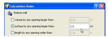
Interactive Schedule criteria now include "Conditional" criteria for certain listing parameters involving the calculation of walls, slabs, roofs, and beams.
