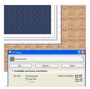
To display surfaces more attractively in 2D views, you can now apply an image fill to any Roof, Slab or Mesh with a cover fill.
