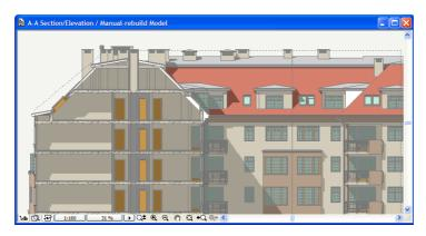
If your Section includes a Distant Area, the same shading options are available in the **Distant Area Options** panel. However, to enable a shading option for the Distant Area, you must first enable the same option type in the **Model Effects** panel. If you disable it in Model Effects, it will become disabled in Distant Area Options, too.
