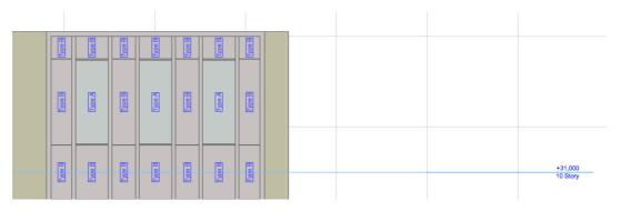
New Inverted Pointer option for labeling in sections: e.g., for displaying the bottom elevation of suspended ceilings
