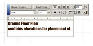
A Text may be started with a double-click while in the Text Tool, (which will result in a "nonbreaking" text block – there are no line breaks, the text block is of flexible width). Alternatively, it may be started by drawing a rubberband rectangle with the Text Tool, which results in a "breaking" text block (meaning the text block's width is fixed, and entered Text will be wrapped to the width of the Text block.) An Editing Window will appear with a Formatting Palette above it.
