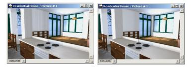
In the following picture you can see effects created by the **SunObject** and **WindowLight** lamp objects. See the light areas on the ceiling of the corridor and the room close to the outside Windows, which is caused by the light generated by these lamp objects.
