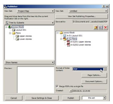
Users no longer need to install a separate PDF driver in order to be able to Publish in PDF from ArchiCAD and PlotMaker.
