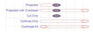
The **Show Projection** field controls how projected multi-story elements should be displayed on each story they are visible on.
